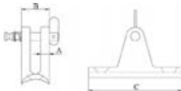
DECK HINGE (RAIL MOUNT WITH REMOVABLE PIN) SS304 OR SS316
