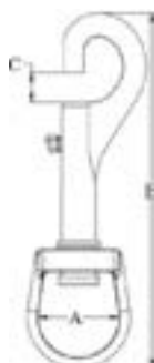
SWIVEL EYE BOLT SNAP SS304 OR SS316
